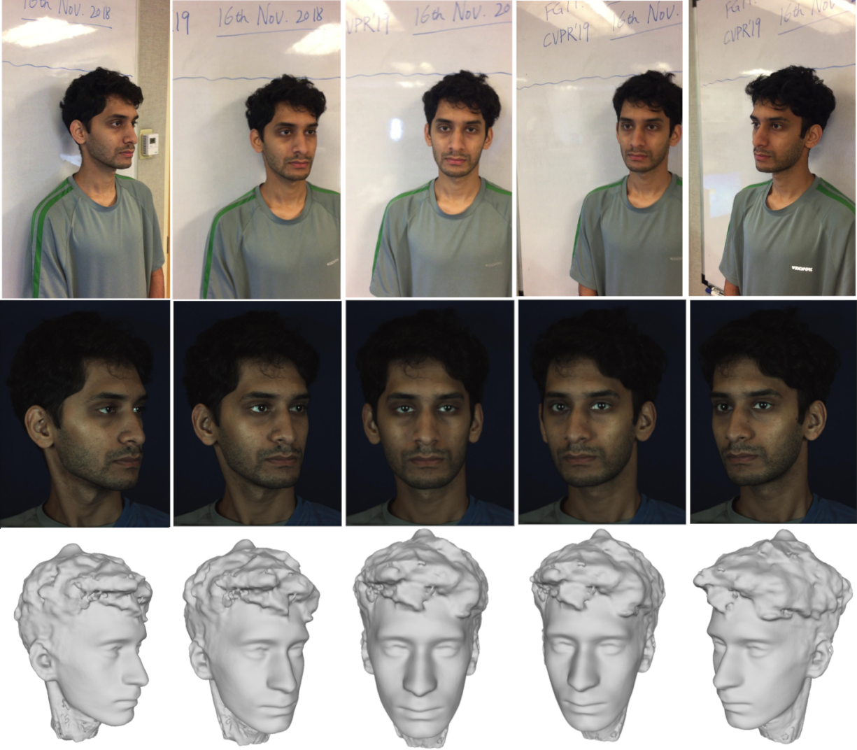
Figure 3.1: (Top) Selected frames from the uncontrolled camera motion, full range video collect on the iPhone 6. (Middle) Selected frames from the controlled camera motion, full range video collect from the DI3D imaging system’s RGB camera. (Bottom) The final ground truth 3D model of the full head of the subject created by merging multiple frame level 3D scans from the DI3D imaging system’s stereo camera.
