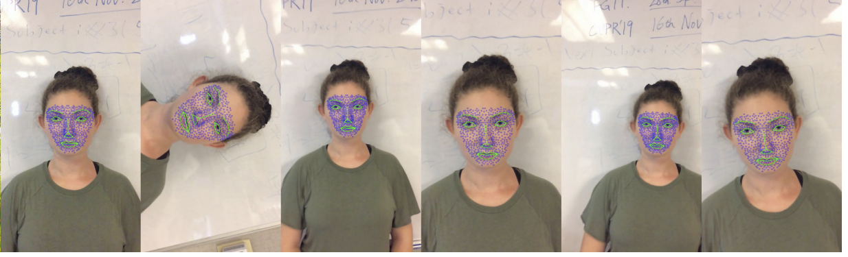
Figure 6.2: The IMU calibration video is collected using the data collection application that also records the IMU data. The IMU video contains quick in-plane rotations followed by back and forward movements to ensure that the signal alignment is accurate, and as shown above tracked with ZFace.
