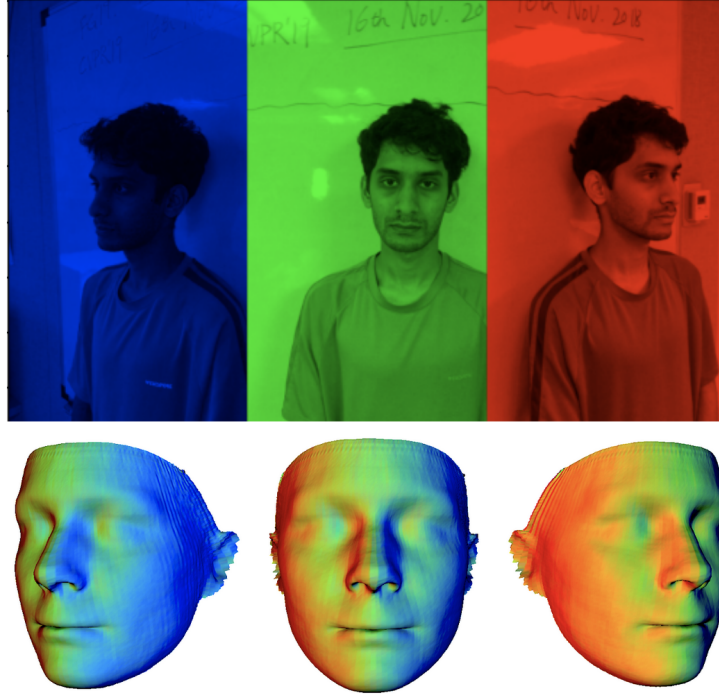
Figure 4.3: The fused mesh from the cosine fusion method color coded to show the combination of the information used from each key-frame.
