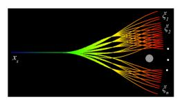
**FIGURE 5** Collision-free paths in a group with an obstacle as the gray dot. The paths start at  $x_s$ . The path ends are considered Monte Carlo samples  $\xi_i$ , i = 1, 2, ..., n, whose distribution is drawn from  $p(x_f|x_s)$  [Color figure can be viewed at wileyonlinelibrary.com]
