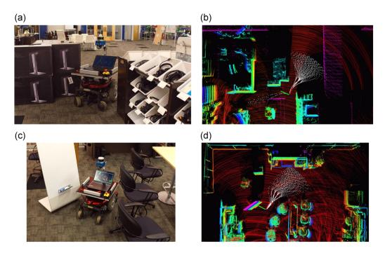
**FIGURE 19** Result of Ground Vehicle Test 2. The vehicle passes through two tight openings as in (a) and (c). (b, d) The corresponding data render where the colored points show the registered scans and the white curves are collision-free paths [Color figure can be viewed at wileyonlinelibrary.com]
