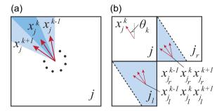
**FIGURE 6** (a) Voxel representation. Each voxel contains multiple directions at a constant angular interval. The state of a voxel is denoted as  $x_j^k$ , j,  $k \in \mathbb{Z}$ , where j is the voxel index and k is the direction index in the voxel. (b) Probability transmission. The probabilities are transmitted to  $x_j^k$  from the adjacent voxels  $j_l$  and  $j_r$  in three directions from each voxel [Color figure can be viewed at wileyonlinelibrary.com]
