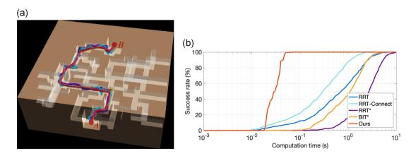
**FIGURE 13** Three-dimensional maze test result. The size of the maze is set at 25 × 25 × 25. (a) An example environment and the paths where all methods generate similar paths. (b) A comparison of the runtime by testing in 50 environments. Given the same success rate, our method outperforms RRT, RRT-Connect, RRT\*, and BIT\* by a factor of 10 in terms of runtime. BIT, batch informed tree; RRT, Rapidly exploring Random Tree [Color figure can be viewed at wileyonlinelibrary.com]
