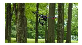
**FIGURE 1** A photo from a flight experiment where our method enables a lightweight aerial vehicle to maneuver at 10 m/s in a cluttered forest environment. More details regarding the experiment are in Section 5.2 [Color figure can be viewed at wileyonlinelibrary.com]
