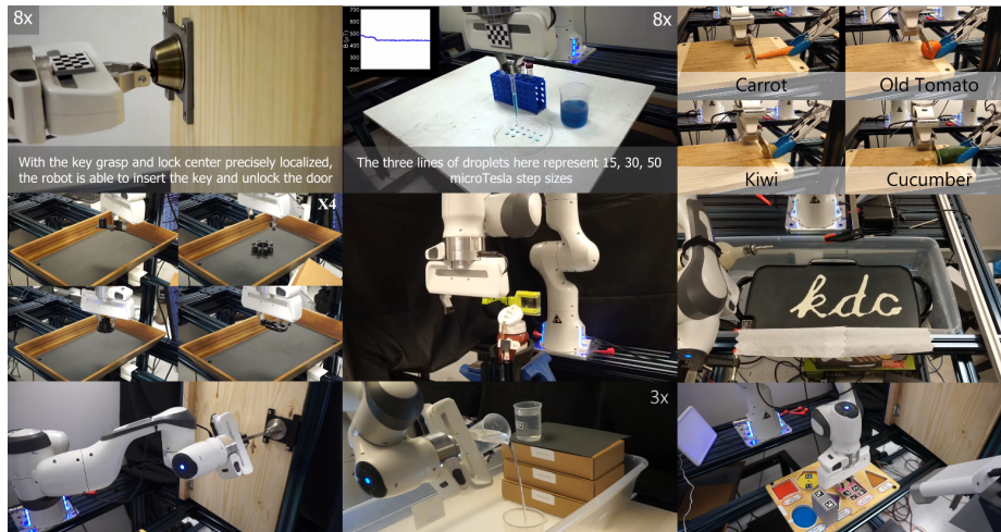
Fig. 1. Collage of Robot Tasks implemented using Franka-Interface and FrankaPy. From left-to-right top-to-bottom, they include unlocking a door with a key, pipetting, cutting vegetables, picking up 3d printed versions of industrial parts, opening a ketchup bottle cap, writing letters using pancake batter, opening a door, pouring water from a beaker, and peg-in-hole insertion.
