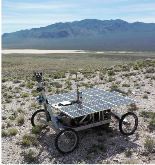
Figure 1: Prototype planetary rover in Cuprite, Nevada exploring terrain to classify and map geology. An on-board spectrometer measures ground spectra to identify mineralogical composition.
