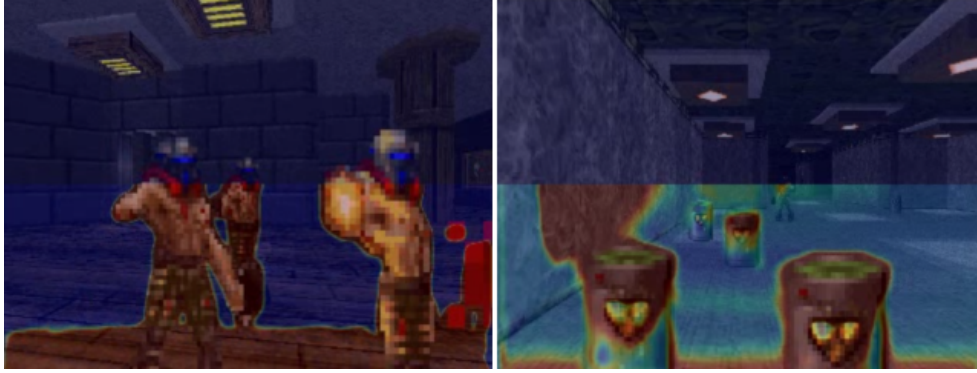
Figure 2.4: Examples of affordance maps \hat{y} predicted by the navigability module, showing accurate localization of semantic constraints within the scene. (Left) contains dynamic hazards in the form of monsters and (Right) contains areas of geometry-affordance mismatch, in the form of barrels shorter than sensor height.
