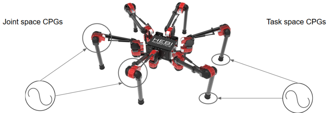
Figure 2.1: Example mappings between CPG oscillators and the actuator space of the robot. The joint space CPG, on the left, maps the output of an oscillator to positions of the joints for each limb. The task space CPG, on the right, maps the output of an oscillator to the motion of the foot of the robots.
