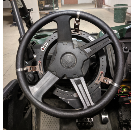
Figure 2.9: Steering actuator as fitted in 2014 Figure 2.10: Current state of steering actuator
