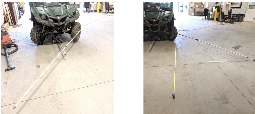
Figure 2.20: Setup used for measuring front wheel steering angle limits
