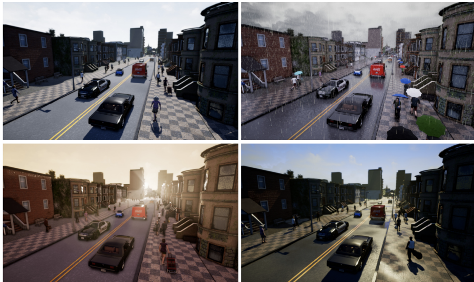
Figure 4.1: CARLA Simulator [29]: A realistic urban-driving simulator this is open-sourced for autonomous driving research. The simulator supports multiple actors, pedestrians, weather conditions and maps that are each configurable in the simulator. Credits: CARLA [29]
