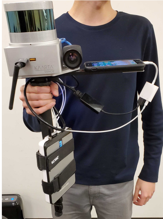
Figure 8: Data collection rig: Seen here is the data collection system, consisting of a LiDAR (upper left), camera (middle), iPhone 8 (right), and battery (bottom). The camera, LiDAR, and computer are part of a commercial Kaarta Stencil SLAM system that we use for ground truth positioning; the IMU signals are recorded using the iOS CoreMotion API.
