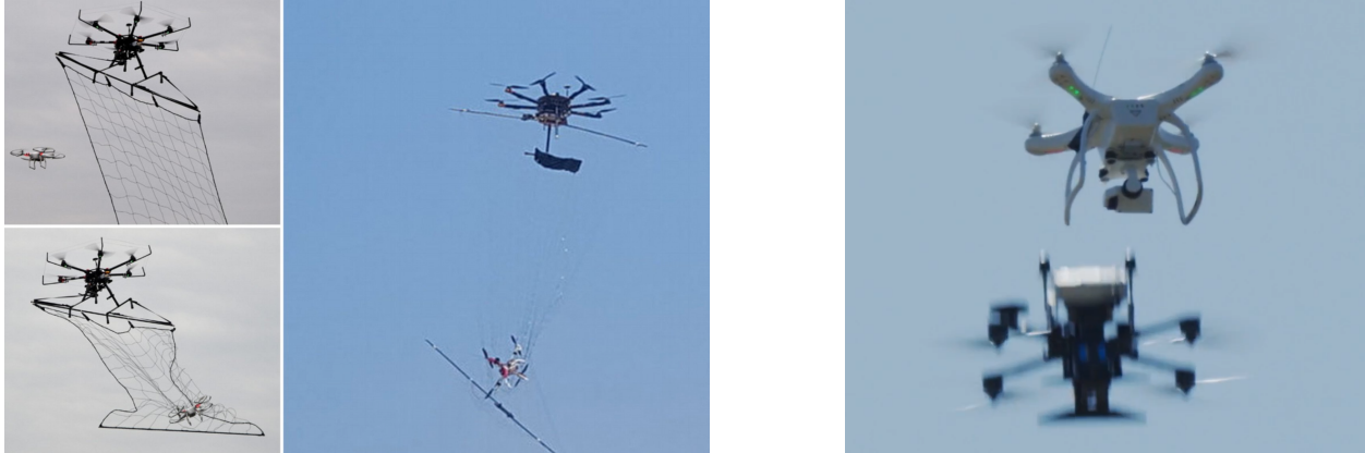
(a) Iterations of the South Korean police counter-UAV aerial system equipped with nets [7].
