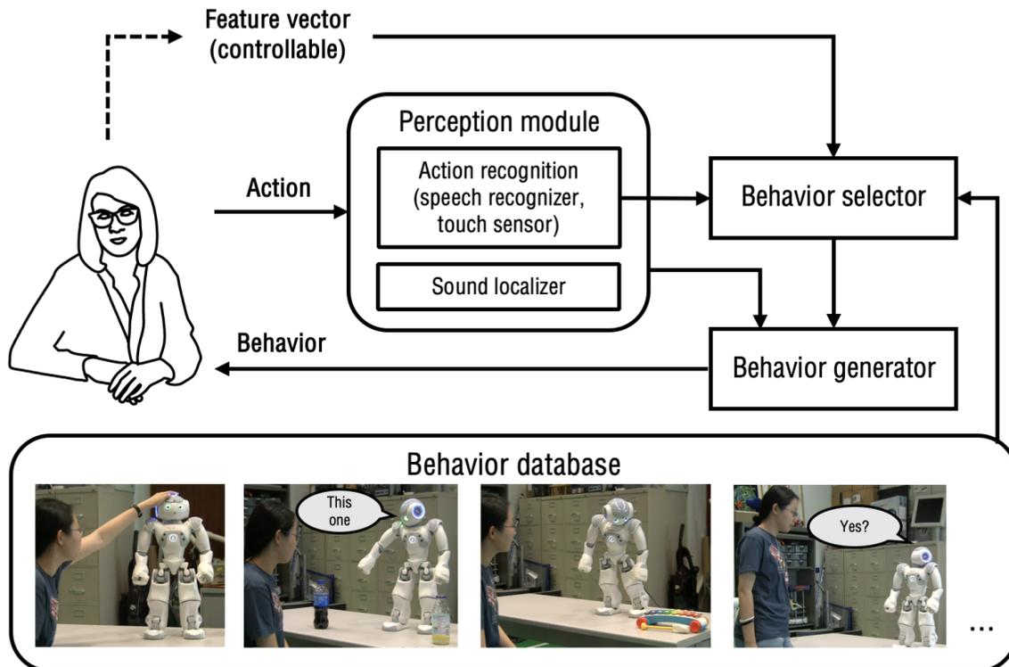
Figure 5.2 Overview of the autonomous robot architecture.
