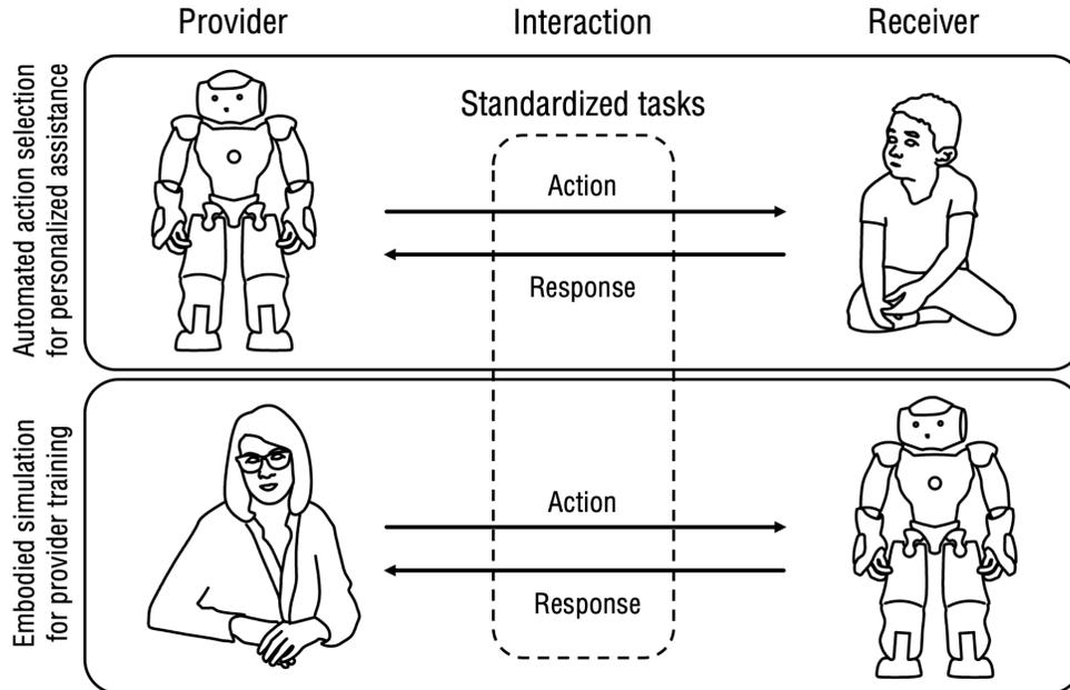
Figure 1.1 Robot-as-provider and robot-as-receiver components of the thesis approach (top and bottom respectively). Standardized tasks are assumed to be similar across the two components, and are modeled as sequences of provider actions and receiver responses.
