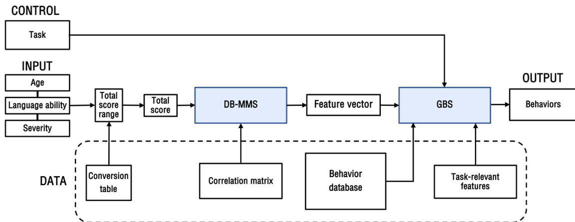
Figure 4.8 Overview of the ADOS-Sim architecture. Algorithm blocks are shown in filled blue to differentiate them from variable blocks.
