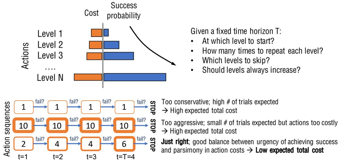
Figure 3.1 Generic example illustrating the concept of optimizing action sequences in relation to given action success probabilities and costs. Numbers in action sequences represent action levels. At every trial, in case of failure the agent continues the sequence, and in case of success gets a reward and aborts execution. Graphs and action sequences shown are only meant for illustrative purposes.
