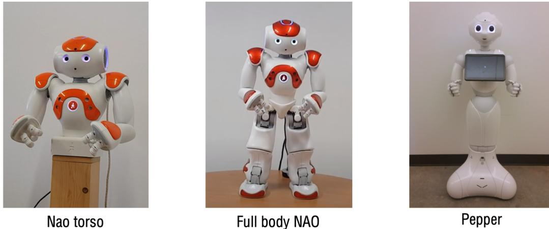
Figure 5.7 Robotic platforms with increasing expressive modalities from left to right.
