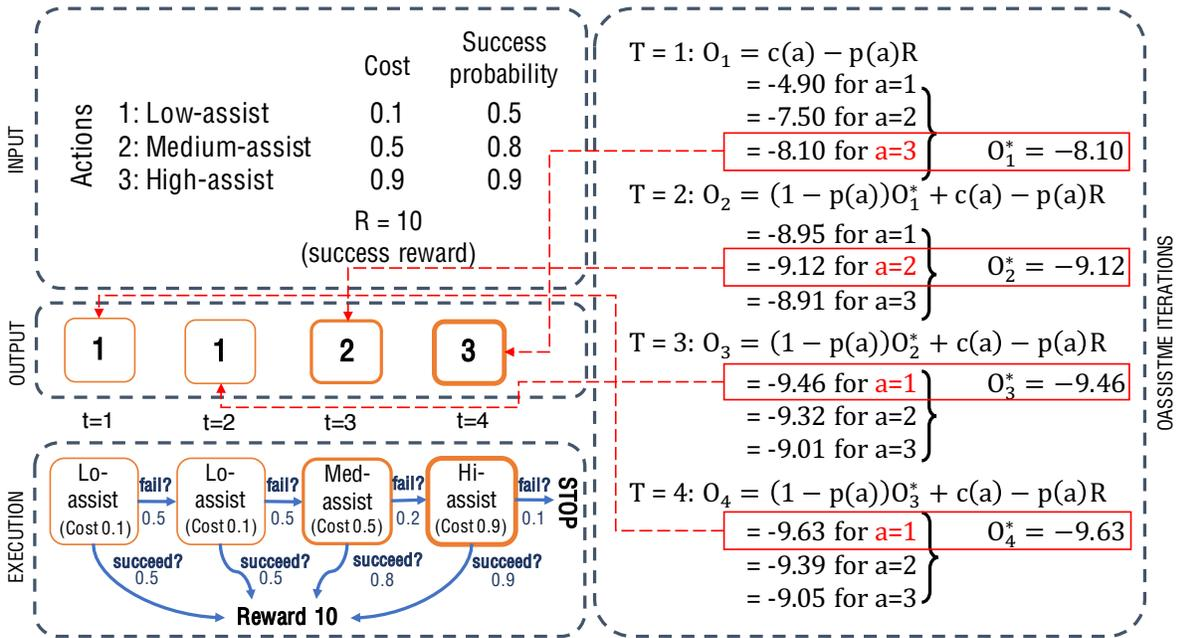
Figure 3.2 Worked example with  $N = 3$ ,  $T = 4$ , and sample action parameters, showing: the computation of the optimal objective at every iteration, the resulting optimal action sequence, and the practical execution of the action sequence by the agent. Numbers below action outcomes represent probabilities.
