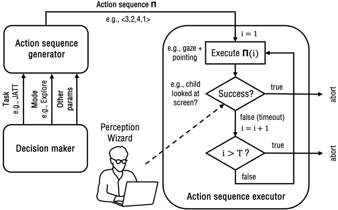
Figure 2.2 Robot control architecture.
