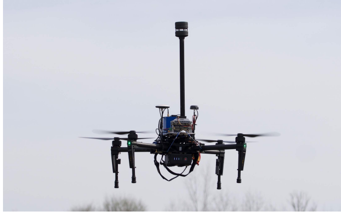
Figure 4.6: The test UAV with the ultrasonic wind sensor.
