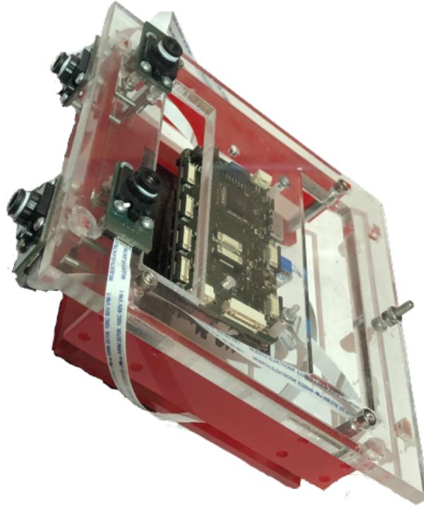
Figure 4.5: The multi-stereo camera rig used to collect experimental results. Images were captured at 25 Hz and inertial data was collected at 200 Hz. All cameras were synchronized using the on-board FPGA.
