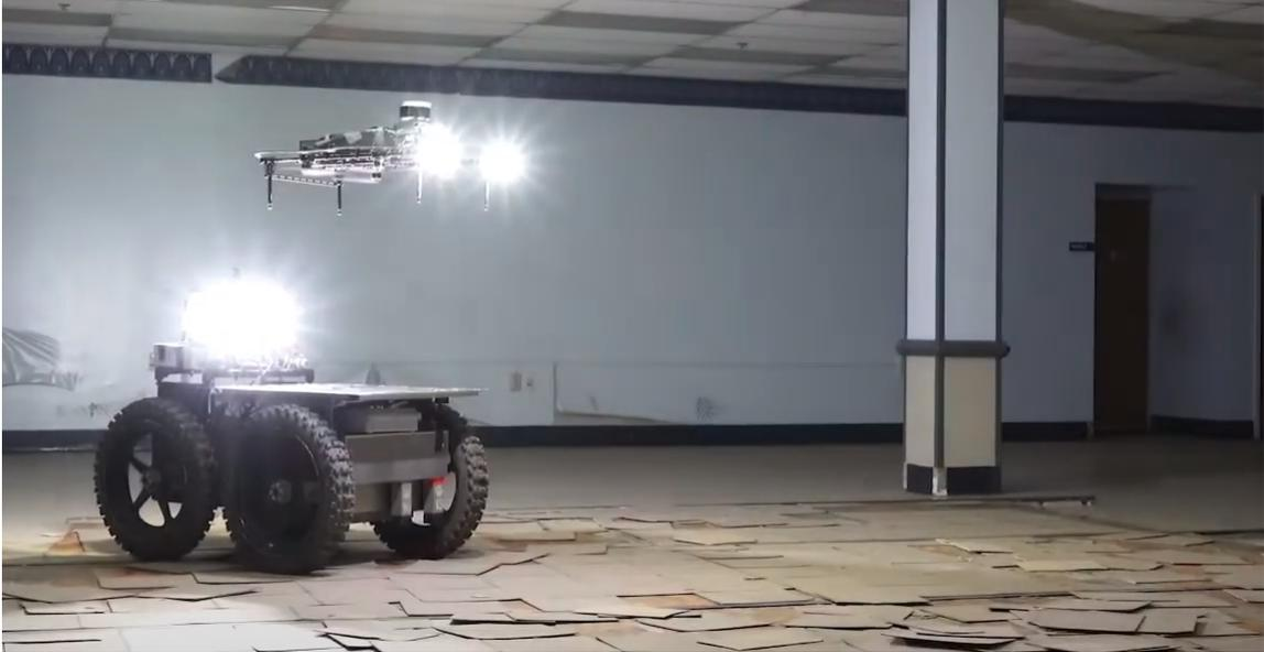
Figure 1.1: One of Team Explorer’s drones taking part in preparation for the DARPA Subterranean Challenge. The drone is tasked with exploring large underground environments in order to perform search and rescue. Being able to rely on vision as the primary means of obtaining a state estimate would obviate the need to carry heavy sensors like lidar and buy crucial minutes of exploration.
