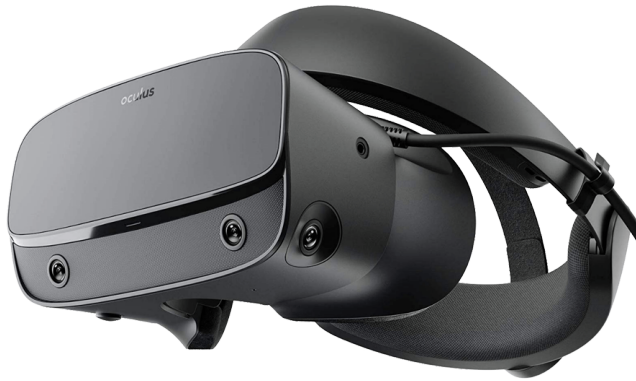
Figure 1.2: Examples of multi camera systems that require extrinsics calibration. ( left ) Facebook Oculus headset with camera sensor facing different directions. ( right ) Drone with two stereo camera sensors [1].
