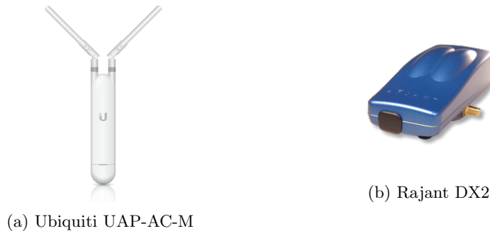
Figure 3.1: Team Explorer communications hardware used in the STIX Event and Tunnel Circuit (a) and the Urban Circuit (b)
