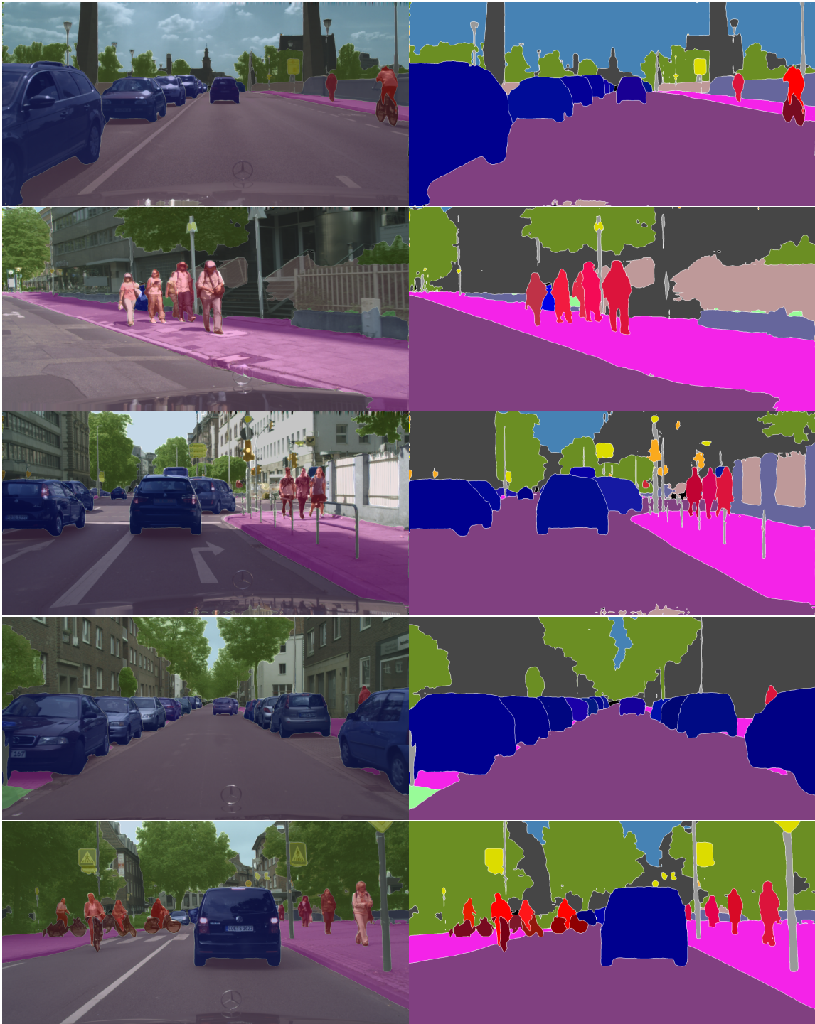
Figure 3.2: Visual prediction of PanoNet on Cityscapes dataset (1 of 2). First column: overlaid results; second column: corresponding panoptic segmentation results.
