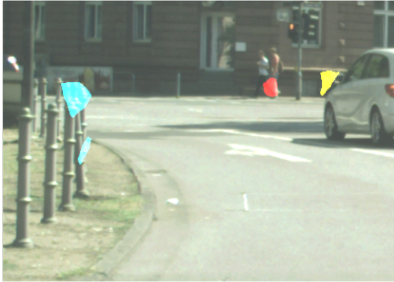
Figure 3.3: Zoomed-in view of mislabeled semantic regions. The highlighted regions are all mislabeled as ‘bicycle’ class by the semantic segmentation branch. They are clustered into three ‘bicycle’ instances, resulting in three false positives.
