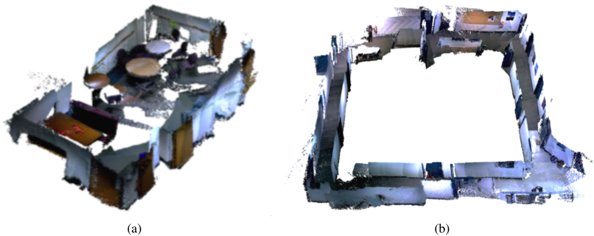
Figure 5.14: Dense 3D reconstruction of various indoor environments using our DPI-SLAM system. (a) An open space with three round tables. (b) Corridors in a loop with lighting changes.
