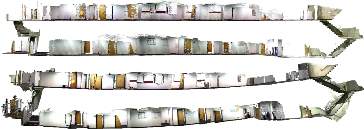
Figure 5.7: Two floor dataset reconstructions by KDP-SLAM (top) and Kintinuous (bottom). Note that KDP-SLAM has reduced drift and maintained the planar structure after loop closure compared to Kintinuous.
