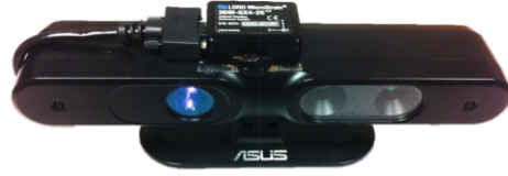
Figure 4.2: The IMU (Microstrain 3DM-GX4-25) is rigidly attached on the top of the RGB-D sensor (ASUS Xtion Pro Live).
