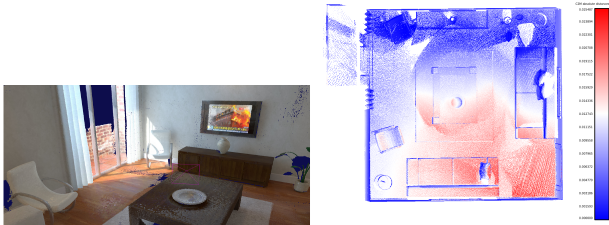
Figure 5.4: Surfel based 3D reconstruction of “Living Room” dataset obtained from ElasticFusion SLAM framework. Right: Surfel centers colored according to their reconstruction error.
