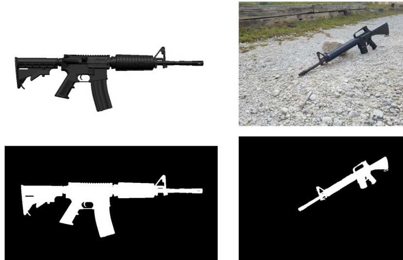
Figure 10: Cutouts of rifles: Upper left is a CAD model of a rifle and on the upper right is a real image of a rifle. Below are the corresponding masks.
