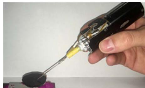
Fig. 1 Micron, an active handheld microsurgical instrument.
