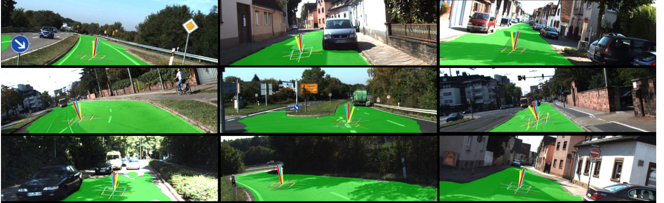
Figure 4: Qualitative results for the ground plane normal estimation. Red: groundtruth. Blue: GroundNet. Yellow: Marr SkipNet. We show that our proposed GroundNet consistently outperforms all other baselines.
