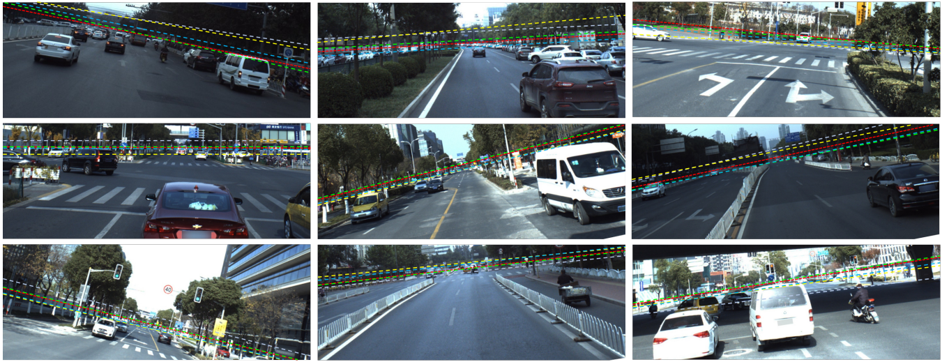
Figure 5: Qualitative results for the horizon line estimation. Red: groundtruth. Green: GroundNet (DSAC). Cyan: Perceptual. Yellow: DeepHorizon. Gray: Zhai et al. We show that our proposed GroundNet consistently outperforms all other baselines.
