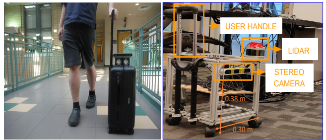
Fig. 2. Left: We show an assistive suitcase with a camera sensor and speaker to guide people. Right: We show the corresponding suitcase-shaped training prototype mounted with stereo camera and LIDAR for data collection.
