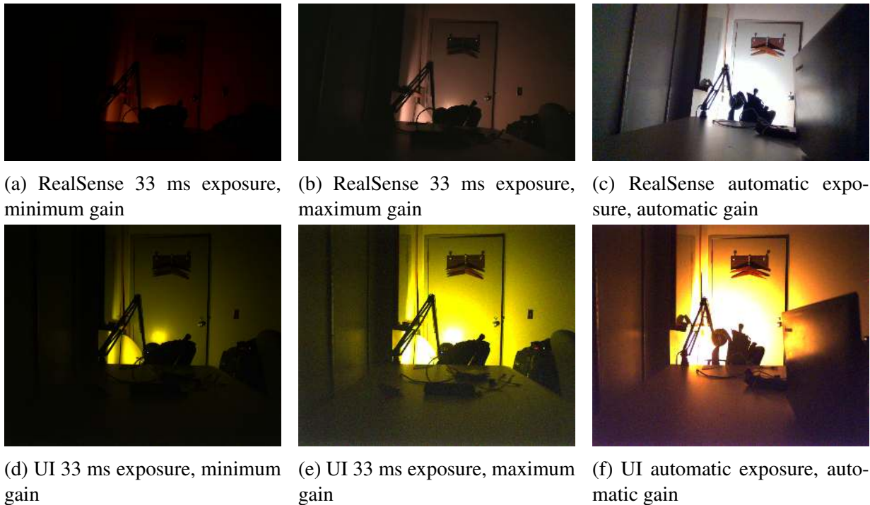
Figure 2.6: Comparison of image quality from UI-3241LE-C-HQ and RealSense D435 RGB cameras across a variety of gain values. Automatic exposure was limited to 33 ms due to a specified framerate of 30 fps for both cameras. It should be noted that after this experiment was performed, it was discovered that the RealSense firmware version used had a bug when setting manual gain which lowered the maximum possible gain value. The automatic gain feature did not have this bug, which could explain why the RealSense image with automatic gain in 2.6c appears significantly brighter.
