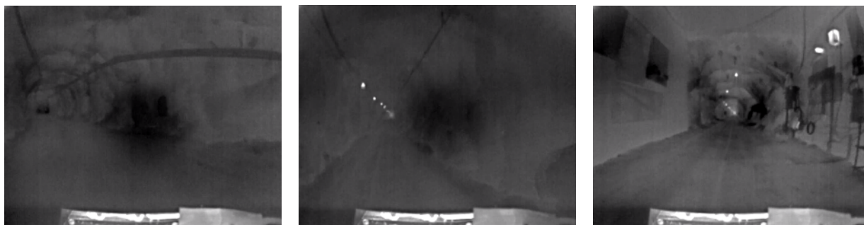
Figure 2.12: The center of each of the 3 images captured from Mk. 0's thermal camera shows an unexpected dark spot. This dark spot is present on images captured from the spares of the same camera model as well, but is not present on the new thermal cameras selected for use in Mk. 1.
