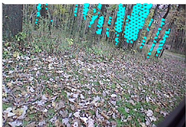
(f) treeBig predictions, VAE 28 Color RBF (cyan = true positives, no false negatives)
