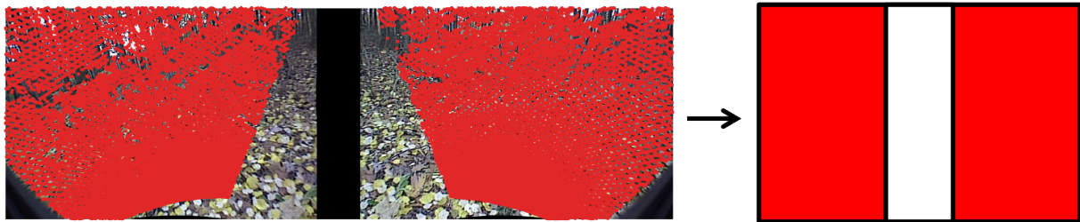
Figure 4.13: Outside the Robot's Path. Left : Wobbler points outside the robot's path, projected onto the image plane. Right : Corresponding short-hand graphic to denote outside the robot's path .
