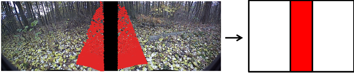
Figure 4.12: Inside the Robot's Path. Left : Wobbler points inside the robot's path, projected onto the image plane. Right : Corresponding short-hand graphic to denote inside the robot's path .
