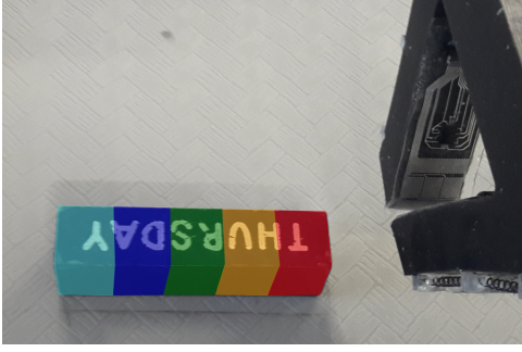
Fig. 9. The grasp location analysis was based on grasps at 5 different locations. These locations (left, semi-left, middle, semi-right, right) are shown in this figure, corresponding to figure 10.
