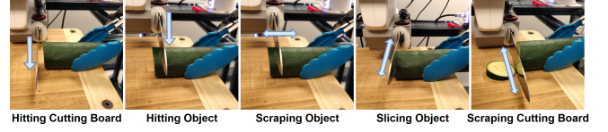
Fig. 5: Different events that may occur when cutting.
