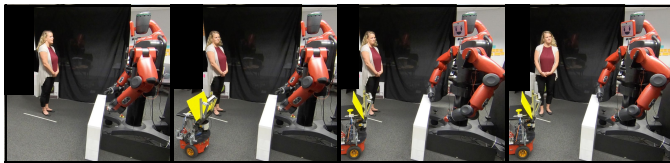
Fig. 4. Example F-formation. Left to right: (1) Participant faces the stationary robot, (2) Mobile robot arrives, (3) Stationary robot turns to talk to the mobile robot, (4) Participant shifts her orientation to ensure a shared space.
