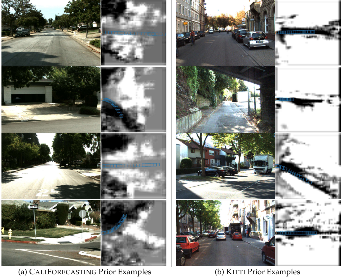
Figure 4.5: The prior penalizes positions corresponding to obstacles (white: high cost, black: low cost). The demonstrated expert trajectory is shown in each scene.
