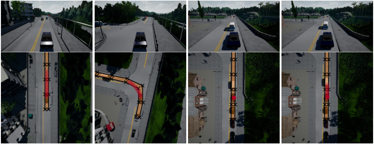
Figure 6.11: Planning with the Region Final State Indicator yields plans that end inside the region. The orange polygon indicates the region. The red circles indicate the chosen plan.
