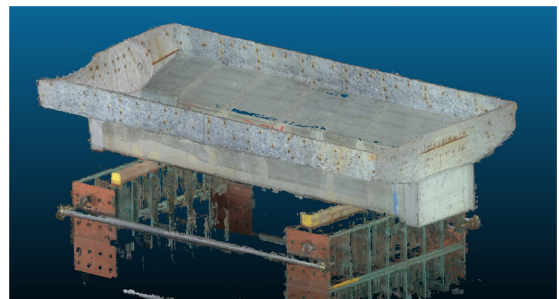
Fig. 7. Built point cloud model of the T-shaped specimen.
