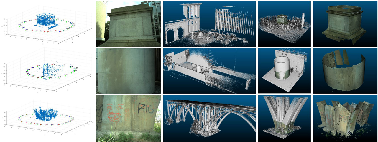
Fig. 9. From top to bottom, the results of three tests are visualized: a squared pillar (top), a cylinder pillar (middle) and a bridge pillar (bottom). From left to right, we visualize the camera poses and landmarks (blue points), a sample of the image data, complete LiDAR point cloud, overlaid LiDAR and stereo point cloud, dense stereo point cloud.
