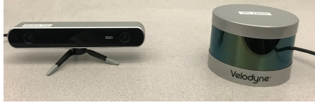
Figure A.2: Velodyne VLP-16 LiDAR and ZED stereo camera used in our experiments.
