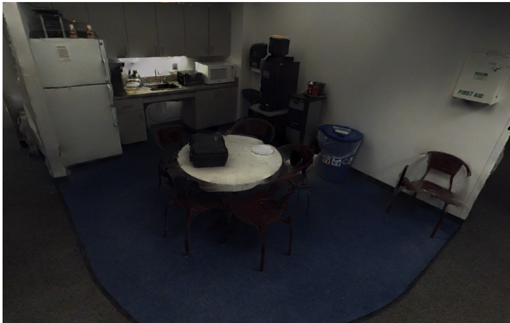
Figure 4.1: Textured mesh without shading from our reconstruction pipeline that exploits the complementary properties of cameras and LiDARs. Our method preserves fine shapes while reconstructing textureless surfaces.
