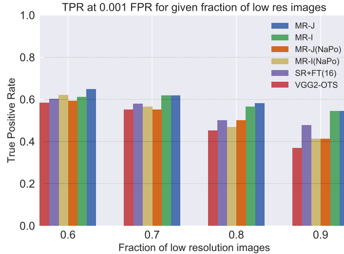
Figure 5.1: Impact of multiresolution pooling The figure shows true positive rate (TPR) at 10^{-3} false positive rate for probe sets with at least 60% low resolution images. The results illustrate that naive pooling, MR-J(NaPo), and MR-I(NaPo), MR features perform worse than multi-resolution pooling, MR-J and MR-I. Interestingly, naive pooling performs worse than SR+FT for probes with large fraction of low resolution images (0.7, 0.8, 0.9), showing that it is sub-optimal to corrupt ‘high resolution features’ from high res images with ‘high resolution features’ extracted from low resolution images.
