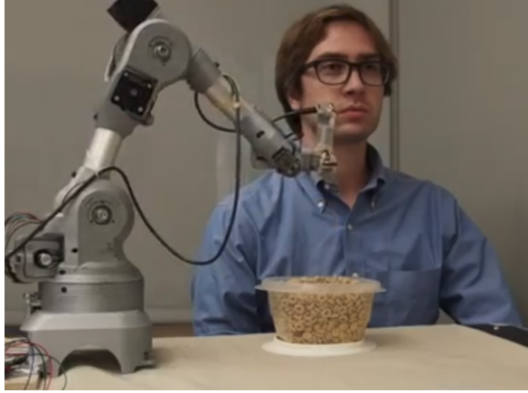
Figure 1.1: The author using a custom-built Niryo One feeding robot running algorithms presented in this work
