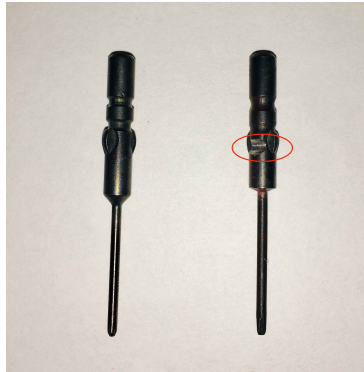
Figure 4.2: Left: rigid-bit, right: flex-bit. The red circle points out the cut slot that makes the screwdriver bit flexible when fixed with a small screw.
