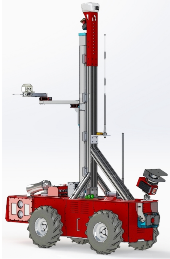
Figure 3.1: Rendering of the ground-based agricultural robot developed at CMU
