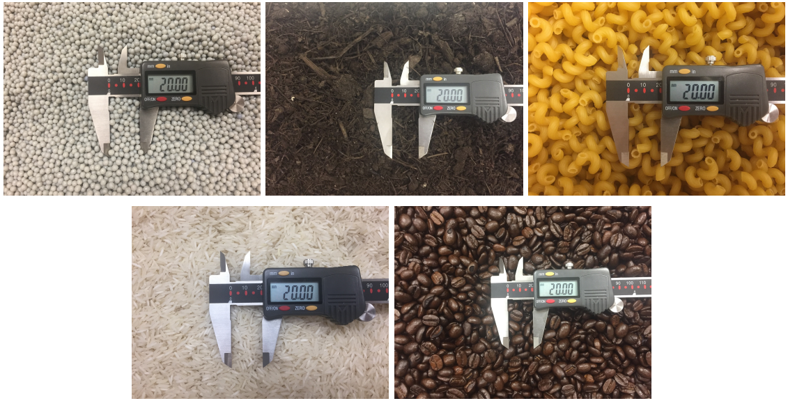
Figure 1.3: The granular materials used in our experiments, with a 2 cm-wide calipers for scale. (Top Left) The plastic injection molding pellets (“Pellets”). (Top Center) The peat moss top soil (“Soil”). (Top Right) The cellentani pasta (“Pasta”). (Bottom Left) The long grain Basmati rice (“Rice”). (Bottom Right) The coffee beans (“Coffee”).
