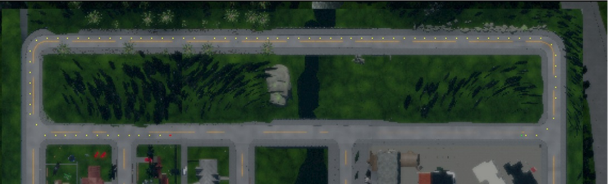
Figure 8.2: Example of proposed CARLA Global Planner providing waypoints (marked in yellow) between start (marked in green) and goal (marked in red) for BIG imitation learning algorithm. As shown in the figure, instead of making a U-turn at the intersection, which is physically not possible due to vehicle’s nonholonomic constraints, or driving backwards, which is not possible due to traffic regulations, the waypoints guide the vehicle towards target in a sequence of left turns, which is the shortest feasible pathway for the vehicle.
