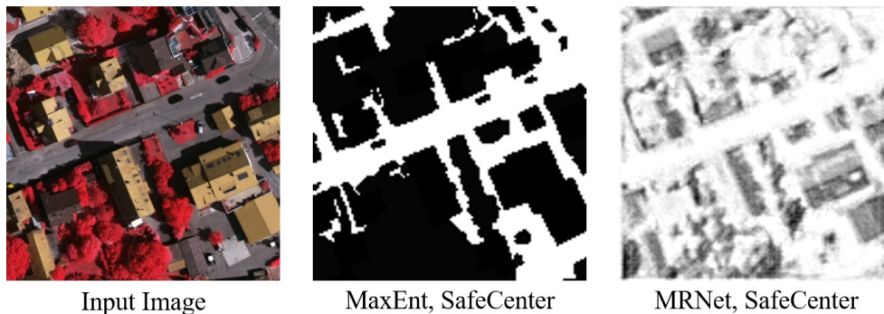
Figure 6.1: Results of SafeCenter training for MAXENT IRL [56] and MRNET. With high cost regions marked in black, we can see that unlike MAXENT where transition between obstacles and driveable space is sharp, MRNET has gradual transition between the two regions, favoring center of the road then edge of roads.
