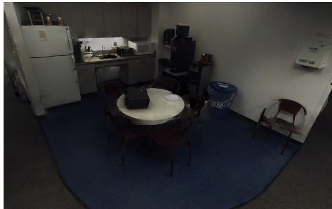
Fig. 1. Textured mesh without shading from our reconstruction pipeline that exploits the complementary properties of cameras and LiDARs. Our method preserves fine shapes while reconstructing textureless surfaces.
