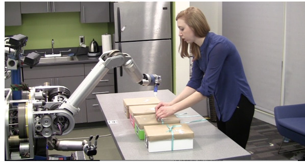
Fig. 4: Participants performed a collaborative gift-wrapping task with HERB to evaluate our reactive goal prediction system against a non-adaptive control and a state of the art predict-then-act system.
