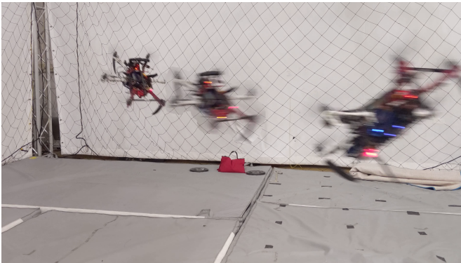
(a) Aggressive trajectory using EPC controller with feedforward terms enabled.
