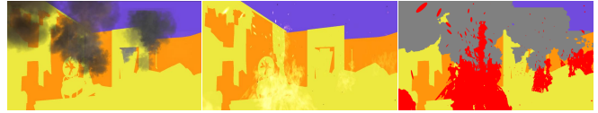
Fig. 6: An example of provided labels for fire cases. Dark gray: smoke (soft label), light yellow: fire (soft label), gray: smoke, red: fire, yellow: furniture, orange: wall, purple: ceiling. The soft label represents a highly detailed transparency-preserving segmentation of flame and smoke.
