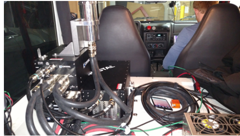
Figure 3.4: Big Vehicle Cloudlet setup in Navlab. The top unit is the pump with coolant, and the bottom unit is the cloudlet.
