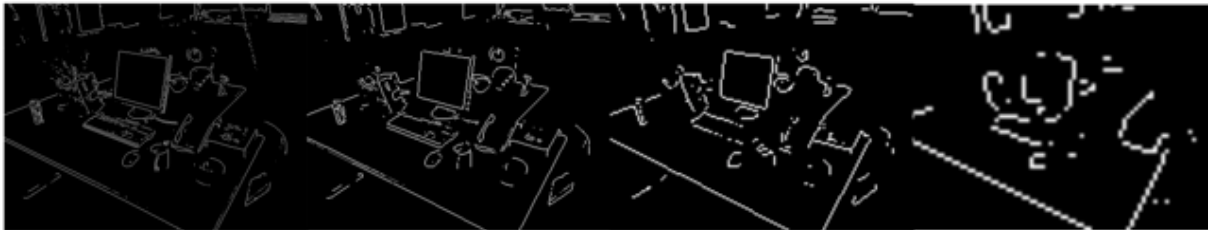
Figure 5.3: Edge pyramid for Canny edges. From left to right: Image 1: 640 \times 480 , Image 2: 320 \times 240 , Image 3: 160 \times 120 , Image 4: 80 \times 60 . Any pyramid greater than three edge images deep starts to suffer from heavy amounts of aliasing, which led us to cut off our edge pyramid at the third level.
