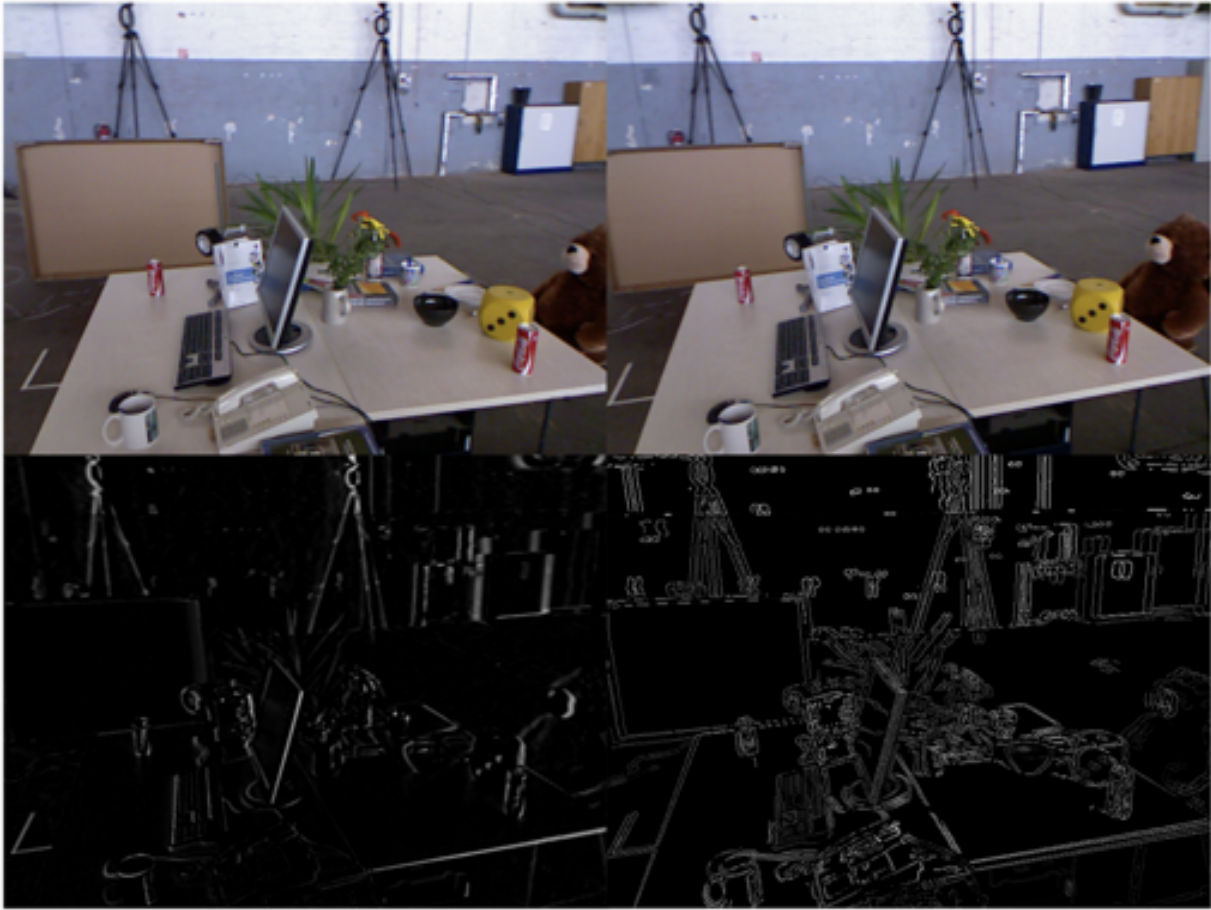
Figure 5.1: In contrast to previous direct methods that attempt to minimize the photometric error (bottom left) between reference frame (top left) and input image (top right), we minimize the photometric error of only the edges (bottom right).
