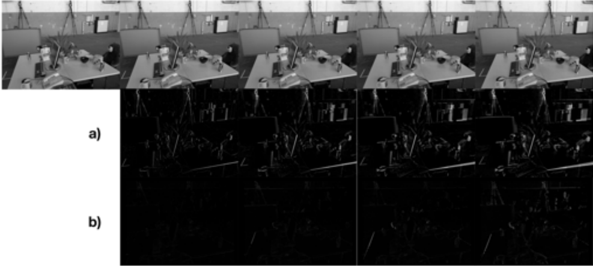
Figure 5.4: In the top row are the original images being localized with respect to the first image. a) All original residuals b) All residuals after only minimizing edge residuals. This shows that minimizing the residuals for just the edge pixels jointly minimizes the residuals for all pixels. After 3 images, the minimization starts to become more inaccurate. This is also a function of camera velocity and rotational velocity.
