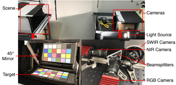
Figure 2. Image Acquisition System. RGB, NIR, and SWIR cameras are co-located using beamsplitters. The target is imaged through a 45° mirror.
