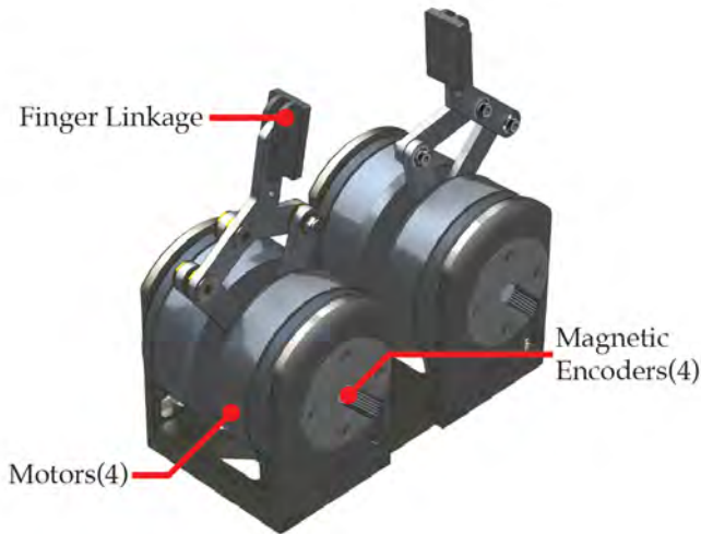
Fig. 5: Design of the two-finger parallel DDHand. The Motor drivers are not shown.
