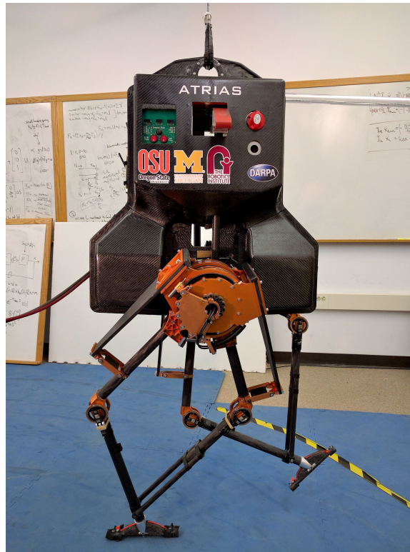
Figure 1.4: We use the ATRIAS biped as a target hardware platform for evaluating our control algorithms. This robot roughly approximates the dynamics of a simplified model due to its light legs and concentrated mass.
