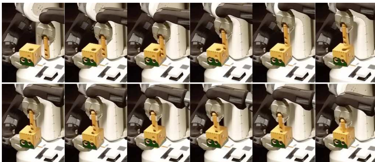
Figure 4.12: Snapshots of a robot experiment for a 2D peg-in-hole task.
