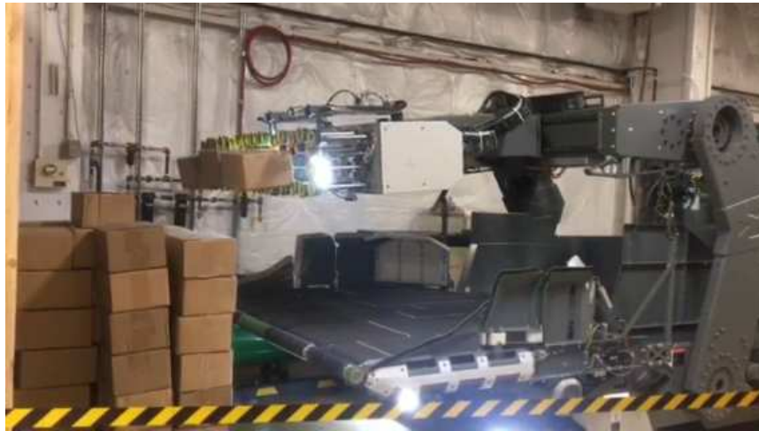
(a) A truck unloader robot is picking up boxes using suction grippers at its arm end-effector.
