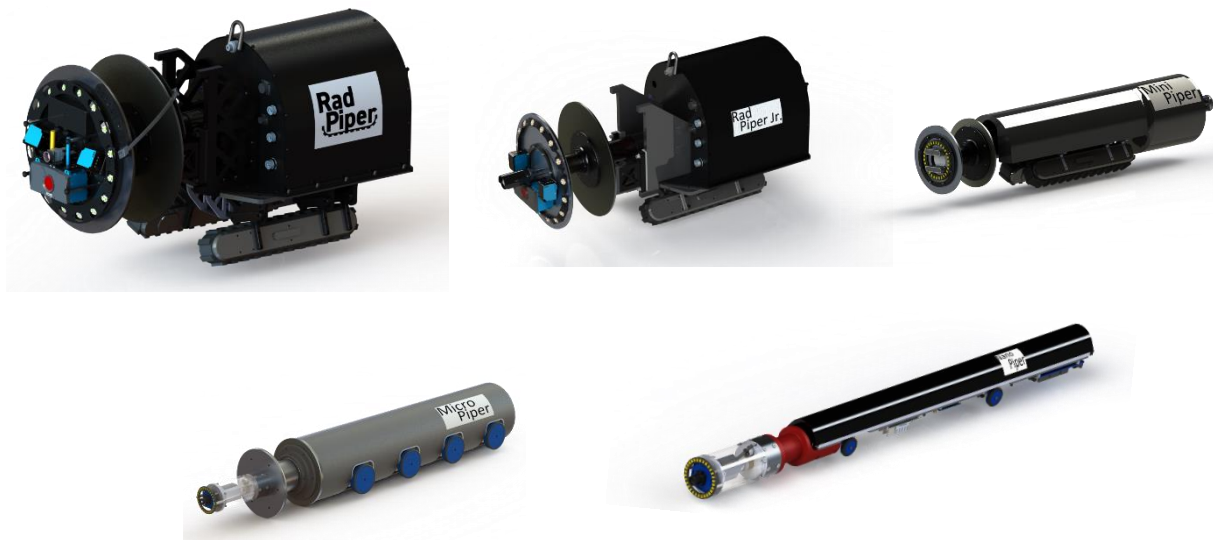
Figure 7: RadPiper (top-left). Concept designs for RadPiper Jr. (top-center), MiniPiper (top-right), MicroPiper (bottom-left) and NanoPiper (bottom-right).
