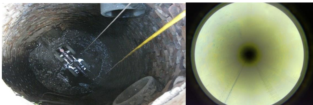
Figure 3: Tethered pipe inspection robot (left). Inside of nuclear piping displaying a distinct lack of features (right).
