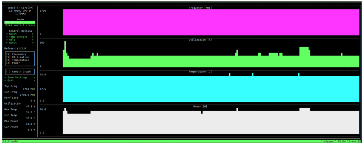
Figure 19: Computer frequency (pink) is at maximum despite less than 100% utilization (green). This leads to increased temperature (blue) and power consumption (gray).
