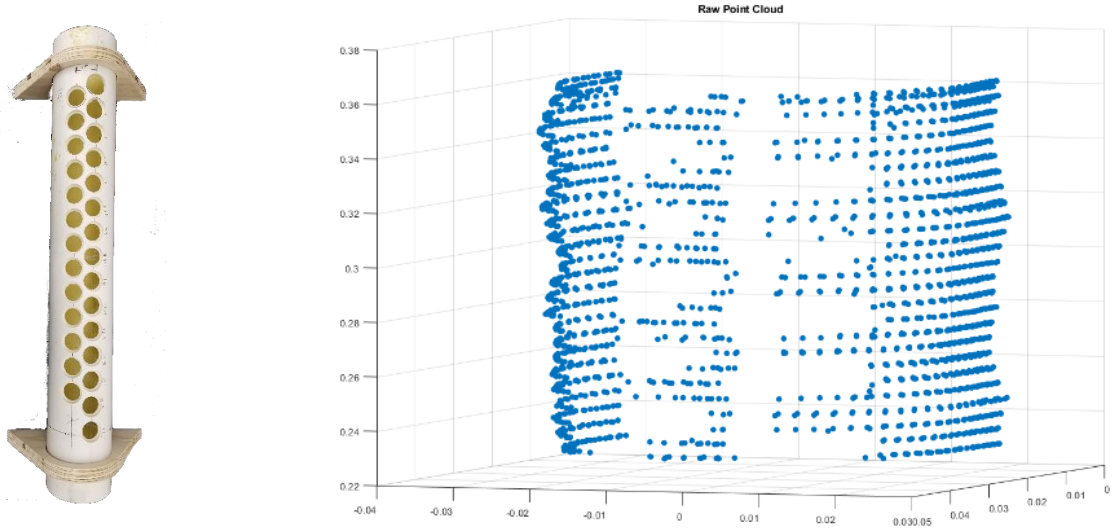
Figure 38: Raw point cloud (right) from 3" piping with drilled holes (left).
