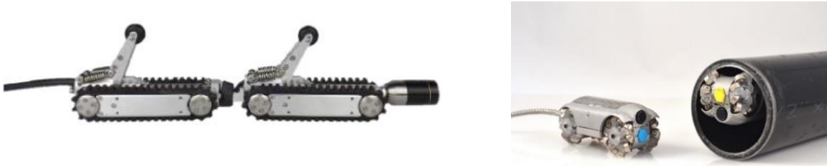
Figure 6: 4" pipe inspection robot from Inuktun (left). 2" pipe inspection robot from HoneyBee (right).
