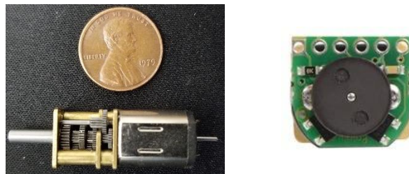
Figure 34: Micrometal gear motor sized 26mm x 10mm x 12mm (left). Optional hall-effect encoder (right).
