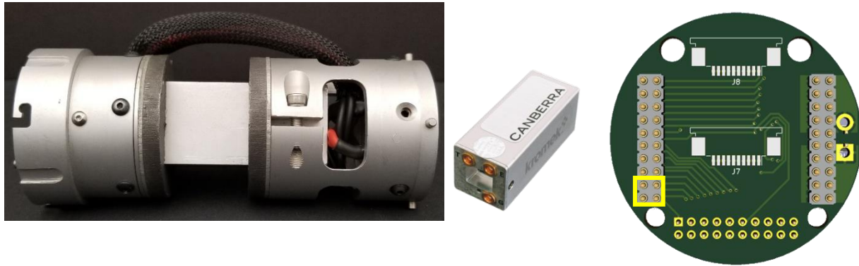
Figure 30: Collimated radiation module (left), with small Kromek CZT detector (center), exposing a USB interface (right).
