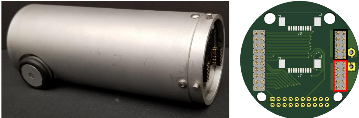
Figure 29: Battery compartment, sized 5.25" in length by 2.22" \varnothing , houses a 42Wh battery at 14V.
