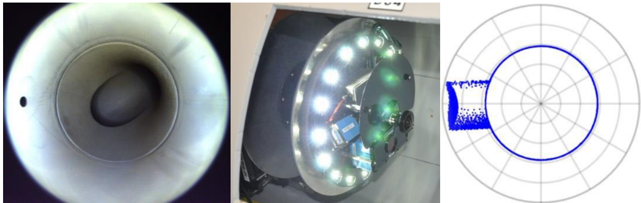
Figure 2: In-pipe imagery (left). Sensor payload (center). Geometric modelling results (right).
