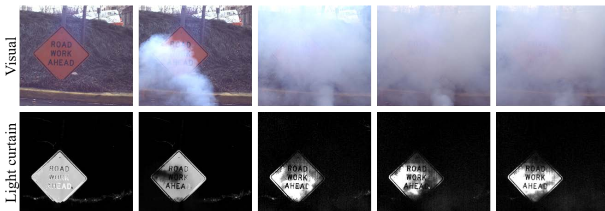
Figure 4.7: Seeing through volumetric scattering media. A fronto-planar light curtain is set at a fixed distance of 5m from the targets in the scene and thick fog is then introduced to the scene. Visibility is highly reduced, but the light curtains suppress multi-path light significantly and can see much clearer.
