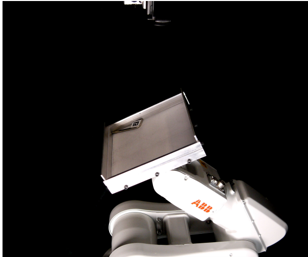
Figure 5.6: Experimental setup. An industrial robot tilts an allen key, with April Tag attached, in an aluminum tray. The overhead camera records the pose of the allen key after each tilt.
