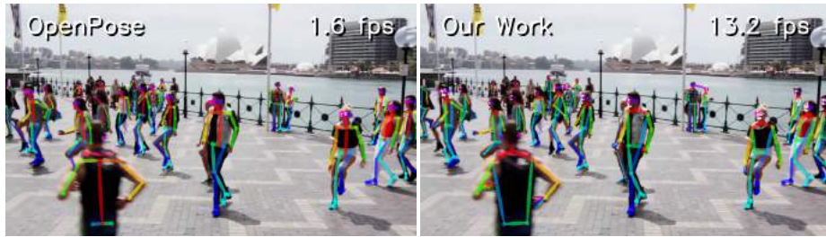
Figure 2: We present the first single-network approach for whole-body pose estimation, with real-time performance that is independent of the number of people in the image. Our work considerably outperforms the current state-of-the-art (our previous work, the original OpenPose [1]) in runtime performance, while it also slightly improves its keypoint accuracy. To avoid confusion, we will denote the original OpenPose as simply “OpenPose”, and our new work as “Our work”.
