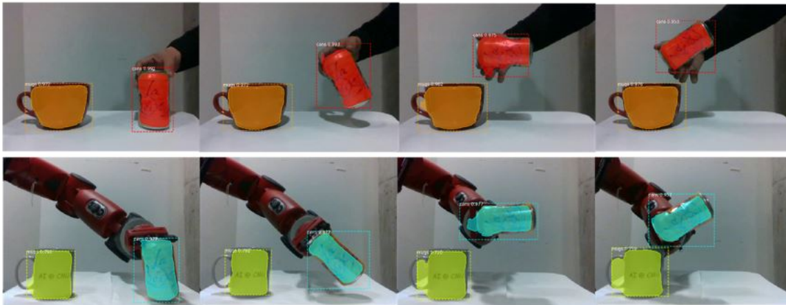
Figure 4.6: Example sequence of detected object entities, mug and can , during demonstration (top) and imitation (bottom).
